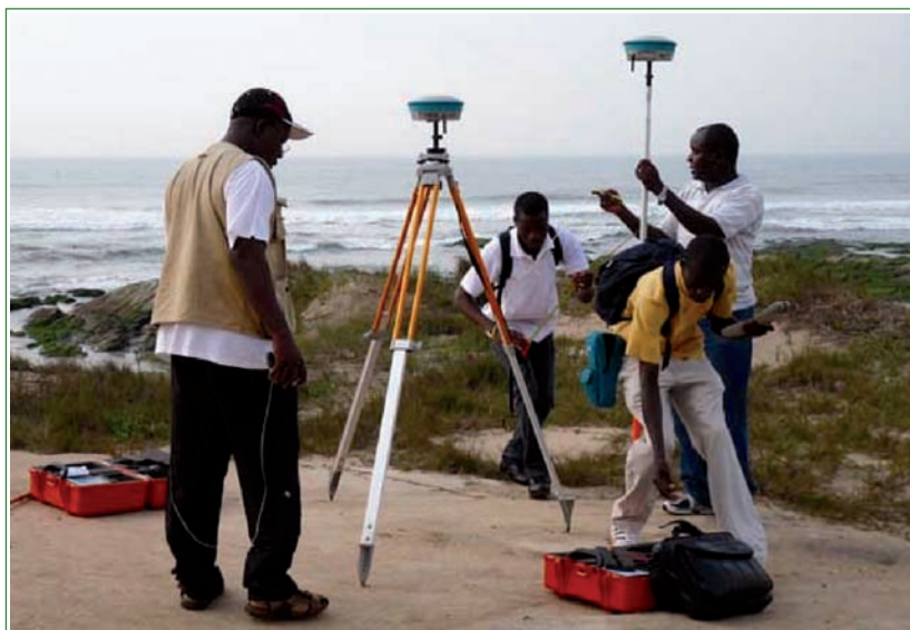
Beach profiling with a high precision global positioning system to monitor coastal erosion
