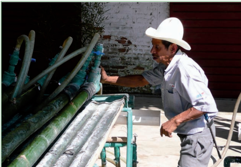
Mexican worker setting up bamboo preservation equipment
