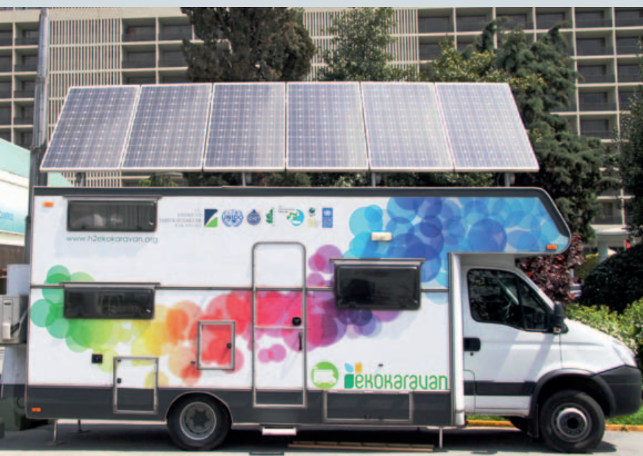
The H2 EcoCaravan attracted considerable attention on its round trip from Istanbul to Vienna for the Vienna Energy Forum. The vehicle—the first of its kind—is a self-sustained living space that runs off wind, solar, battery and hydrogen energy systems. It is a joint demonstration project run by the International Centre for Hydrogen Energy Technologies (ICHET) and the Natural Gas Vehicles Association. ICHET is a UNIDO project founded in Istanbul in 2004 and supported by the Turkish Ministry of Energy and Natural Resources. Its role is to support, demonstrate and promote viable hydrogen energy technologies, with the aims of enhancing future economic development, particularly in emerging countries and preventing the widening of the energy and technology gap while helping to skip over the fossil fuel phase. Photo: UNIDO
