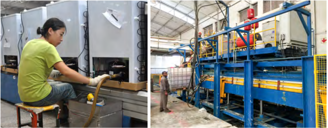
Left: Refrigerator compressor production company in Hubei province, China. These compressors are based on hydrocarbon refrigerants, R600 or R290. Besides protecting the ozone layer and having nearly zero global warming potential, they offer better energy efficiency results than previous CFC12 compressors or other alternatives such as R134a and R404a. Right: A demonstration Montreal Protocol project in South Africa on the technical and economic advantages of vacuum-assisted foam injection in the insulation of discontinuous sandwich panels.
