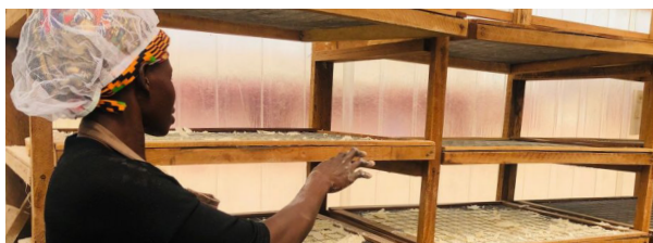
A cassava processor using simple Solar Dryer constructed for JOSMA by UNIDO for its cassava chips which would be further processed after drying
